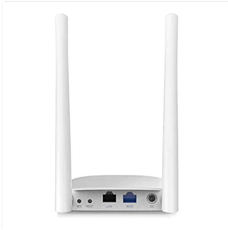
Figure 2: Rear view of the D-Link DIR-811N router, displaying the WPS button, Reset button, LAN port, WAN port, and DC power input.
