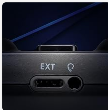
Image: A close-up view of the EXT port and the 3.5mm audio jack located on the bottom of the DR1TECH Shock Pad controller.
