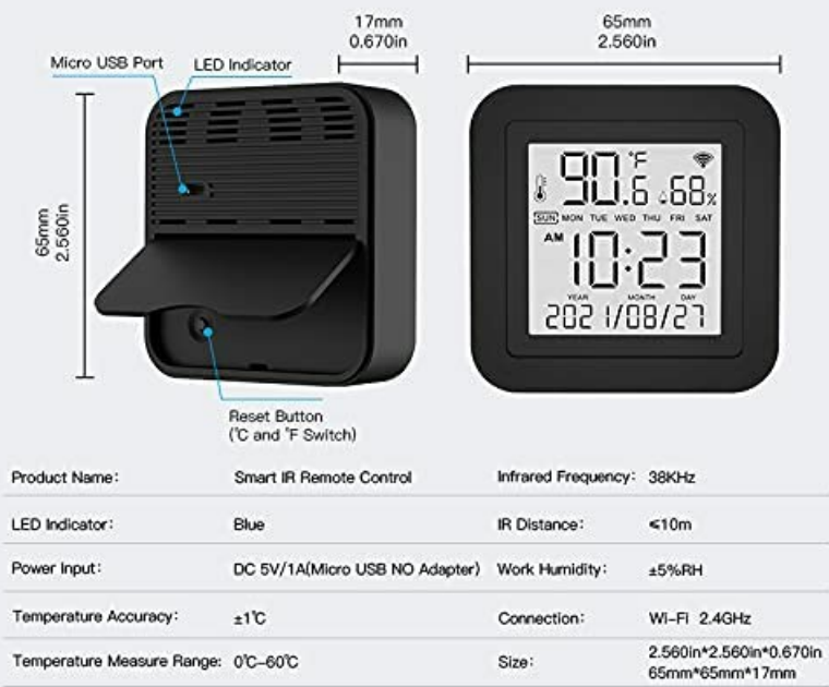
Image 3.1: Product dimensions and component labels for the MOES Smart Temperature Humidity Monitor.
