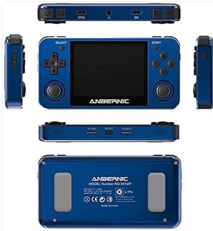
Figure 4.2: Console Layout. This image provides various angles of the console, highlighting the L1/L2/R1/R2 shoulder buttons, OTG and DC ports on the top, volume controls on the side, and TF/EXT, Reset, and TF2/EXT slots on the bottom.
