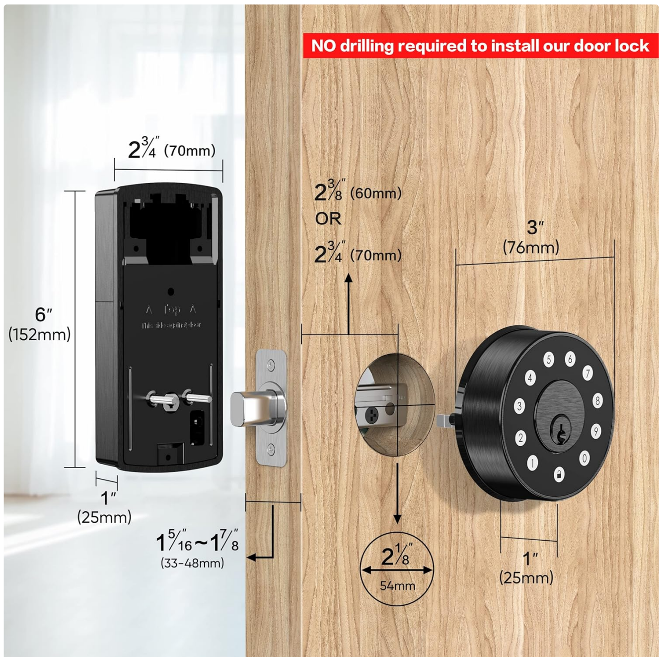
Image: Diagram illustrating the required door dimensions for installing the Sifely Smart Deadbolt.
