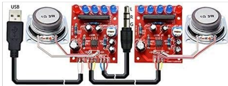
Image: Detailed wiring diagram illustrating how to connect the USB power, 3.5mm audio input, circuit boards, and speakers.
