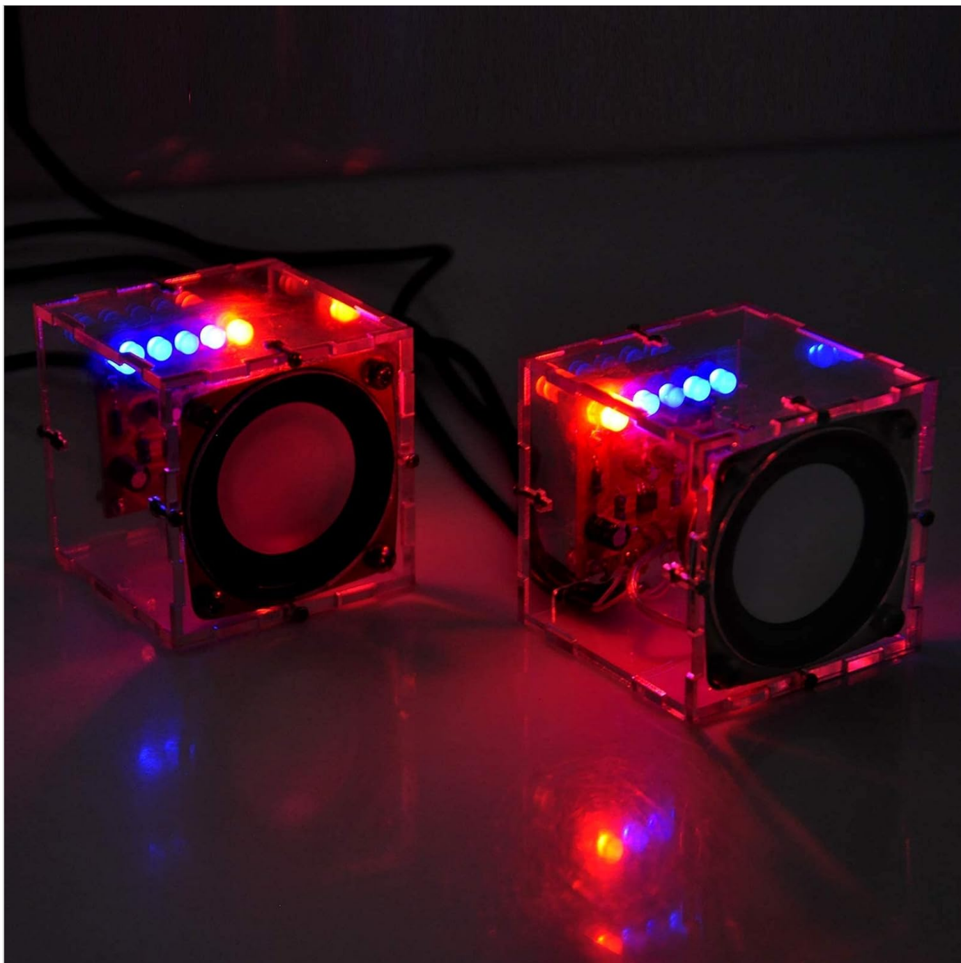
Image: Fully assembled stereo speakers with transparent acrylic enclosures and illuminated LEDs.
