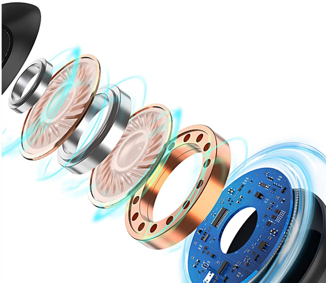
Figure 1: Internal speaker structure for clear sound reproduction.
