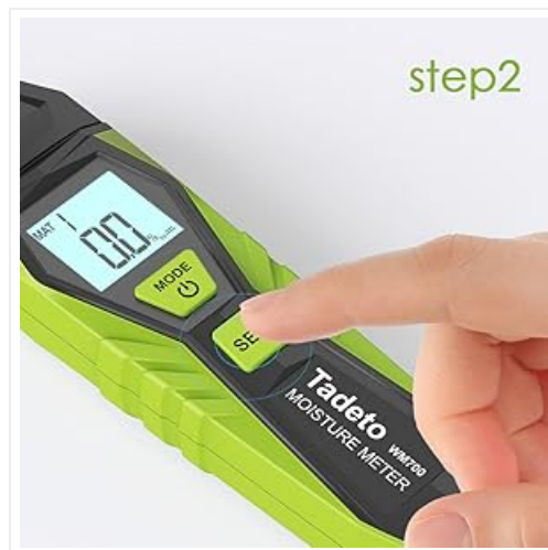
Figure 5: Selecting the material measurement mode (MAT) using the SET button.
