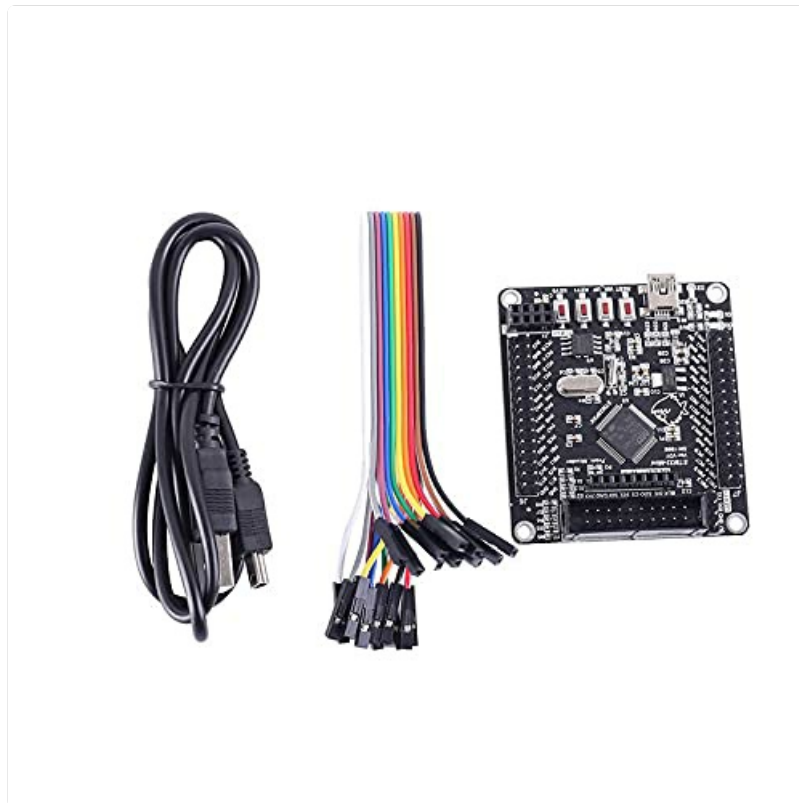
Figure 3: Image showing the STM32F405RG Development Board along with the included Dupont line and USB data cable.
