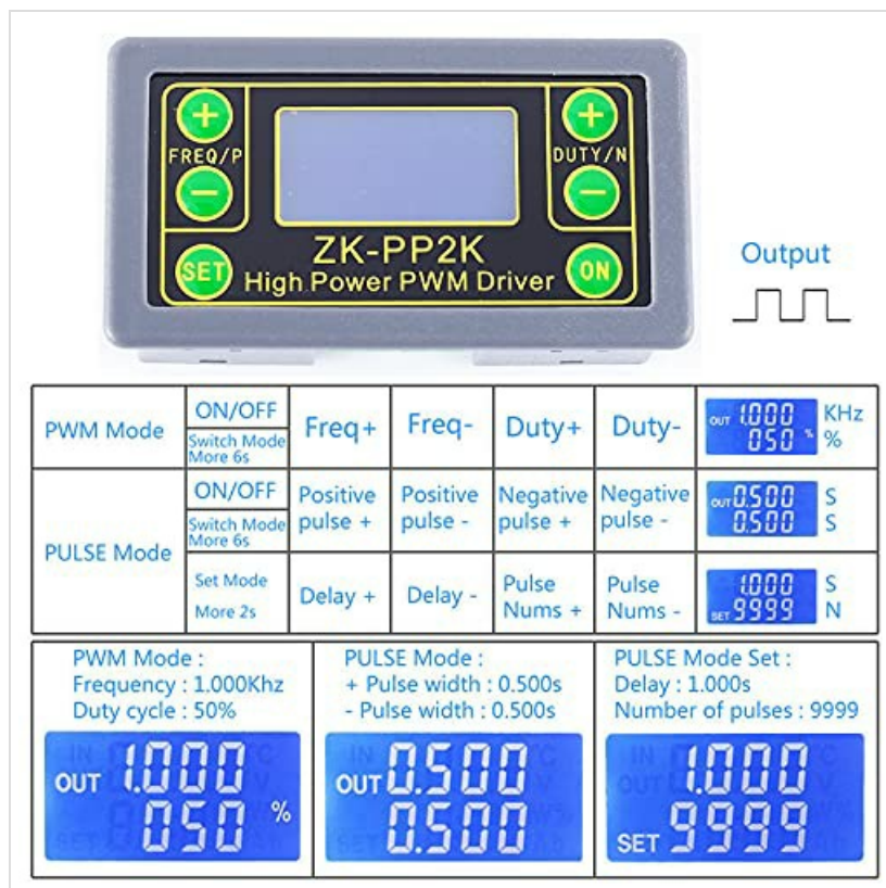
Figure 5.3: Mode Comparison and Button Mapping. This image provides a detailed overview of button functions across PWM and PULSE modes, along with example LCD displays for each mode. It shows how to switch modes and adjust parameters like frequency, duty cycle, positive/negative pulse width, delay, and number of pulses.
