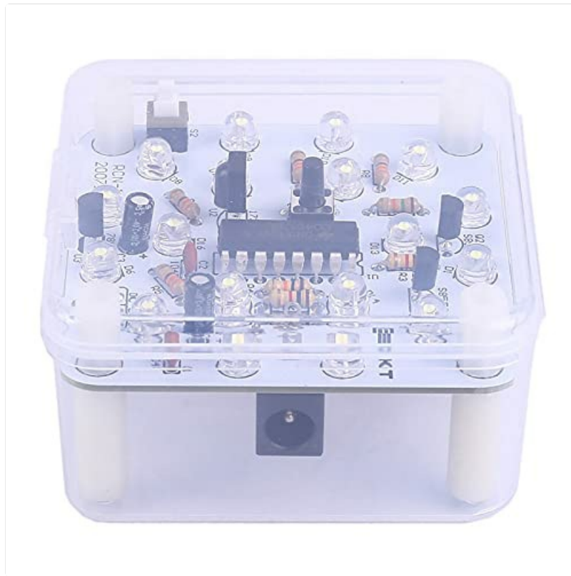
Image 3: Rear view of the assembled RCN-1 unit within its protective casing, showing the 5.5mm power input socket.
