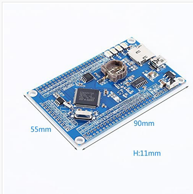
Image 9.1: Diagram showing the physical dimensions of the STM32H750VBT6 Development Board: 90mm length, 55mm width, and 11mm height.
