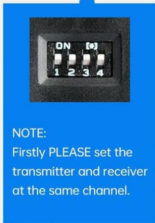
Image 3.2: Diagram illustrating the DIP switches on both the transmitter and receiver for setting the communication channel.
