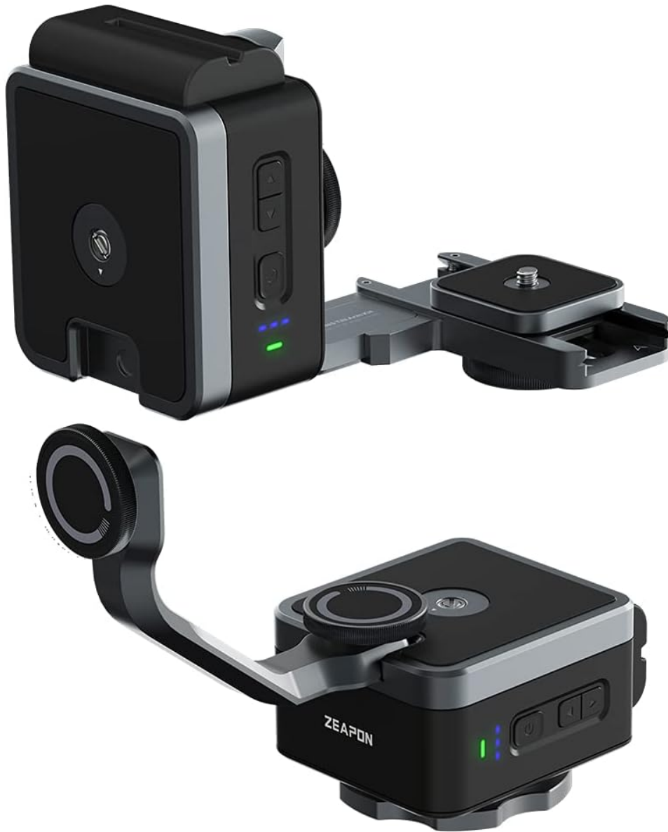
Figure 4.3: The PONS PT module, formed by two PONS units, enabling pan and tilt movements.
