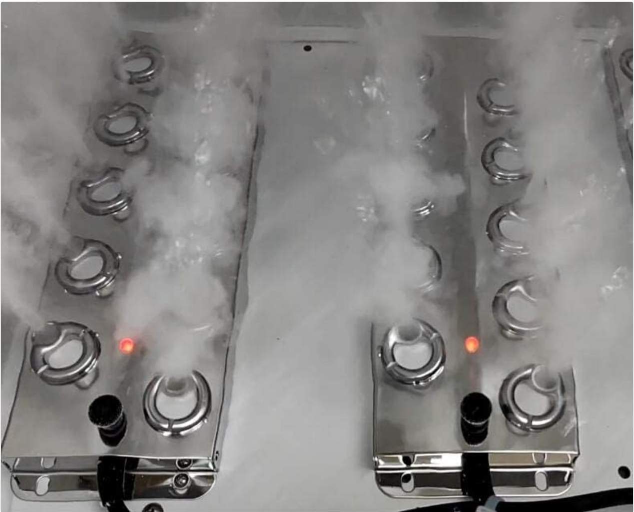
Close-up of the stainless steel mist makers actively producing fine mist, with red indicator lights visible.
