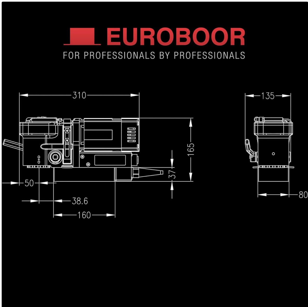
Image 5: Technical drawing illustrating the dimensions of the EUROBOOR ECO.36+ magnetic drill press.
