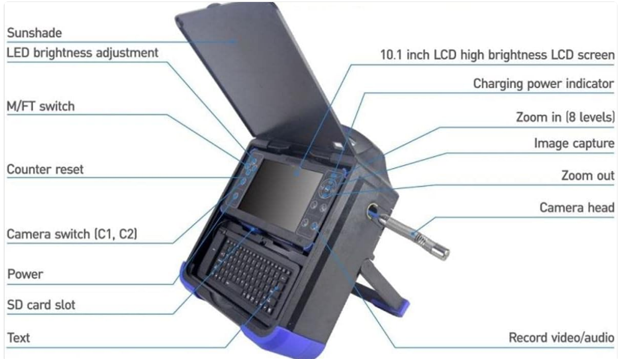
Figure 4.1: Labeled diagram of the Vividia VS-92530 Plus control unit. This image clearly indicates the location and function of various controls, including the 10.1-inch LCD screen, sunshade, LED brightness adjustment, M/FT switch, counter reset, camera switch (C1, C2), power button, SD card slot, text input keyboard, charging power indicator, zoom controls (8 levels), image capture button, zoom out button, camera head connection point, and record video/audio button.
