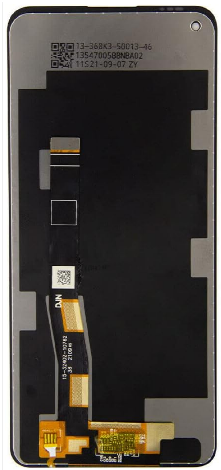
Image 3.1: Rear view of the display assembly, highlighting the delicate flex cables and connectors that interface with the device's motherboard. Handle these components with extreme care during installation.
