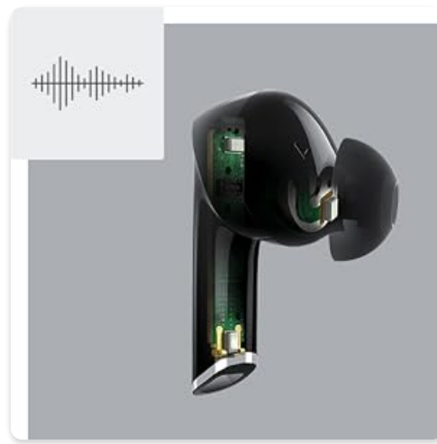
Image: An internal view of a Denon AH-C830NCW earbud, demonstrating the sophisticated components responsible for active noise cancellation.
