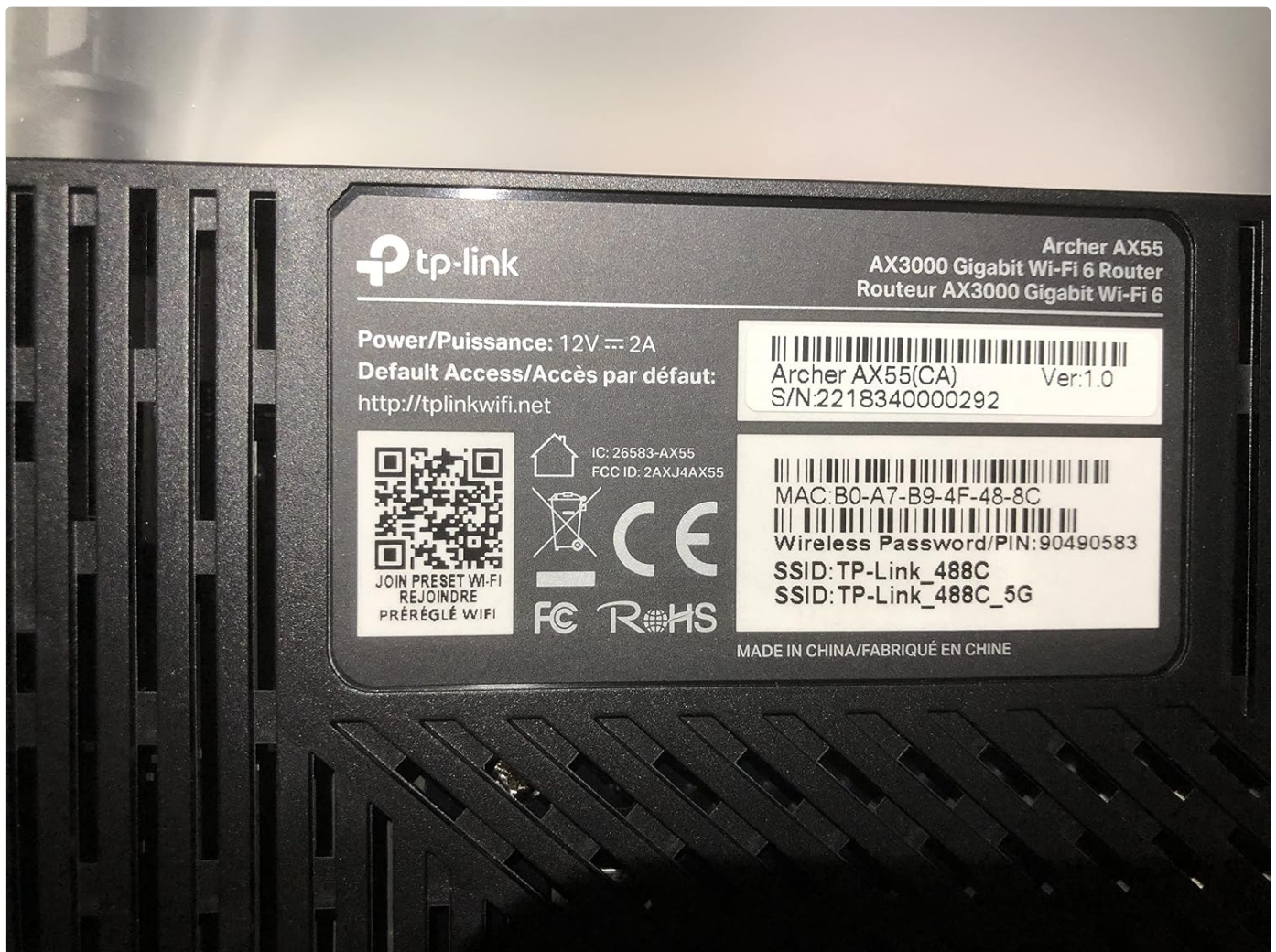
Figure 3: Bottom label of the Archer AX55 with default Wi-Fi credentials and QR code.
