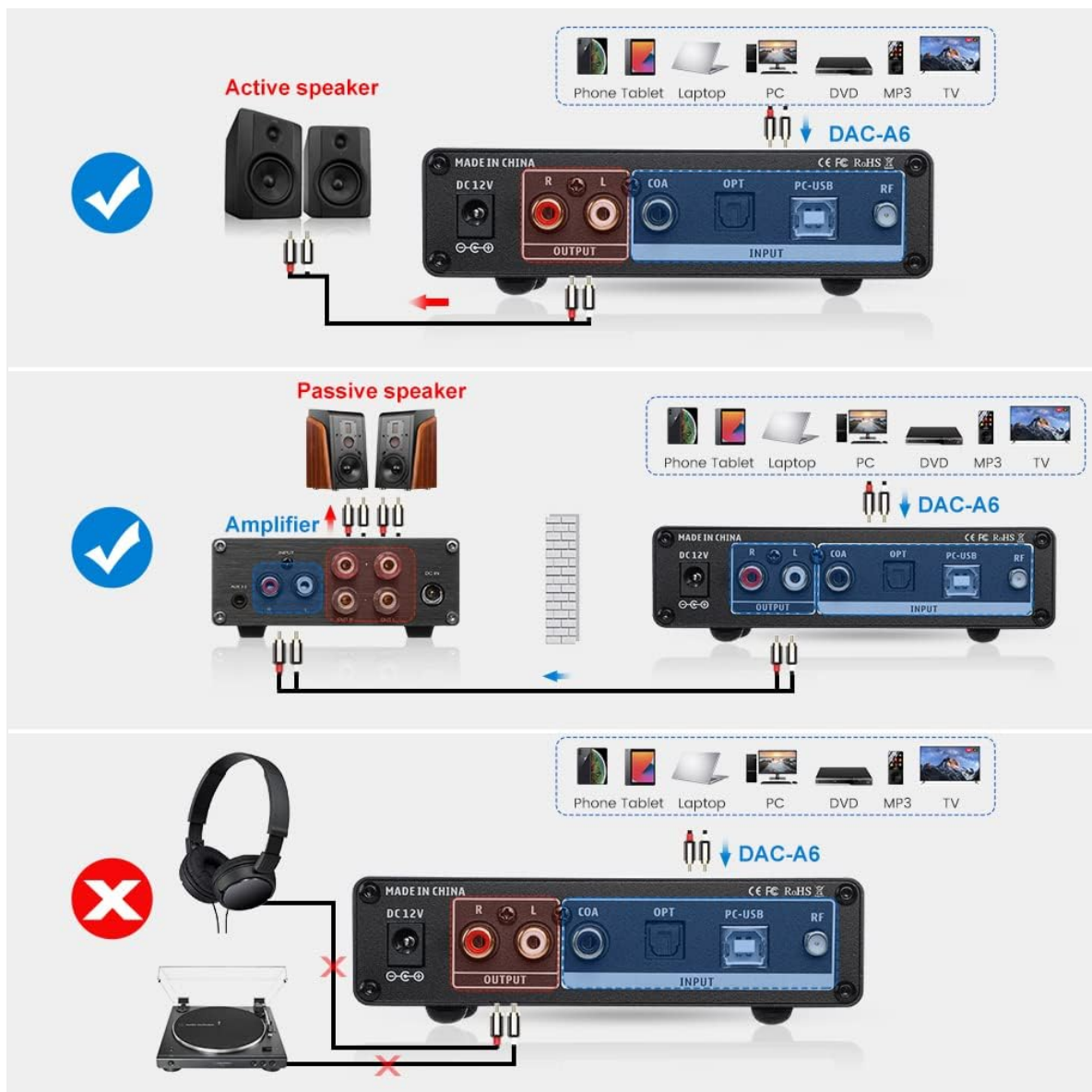
Image: Diagram illustrating connection options for the DAC A6 to active speakers or an amplifier with passive speakers.
