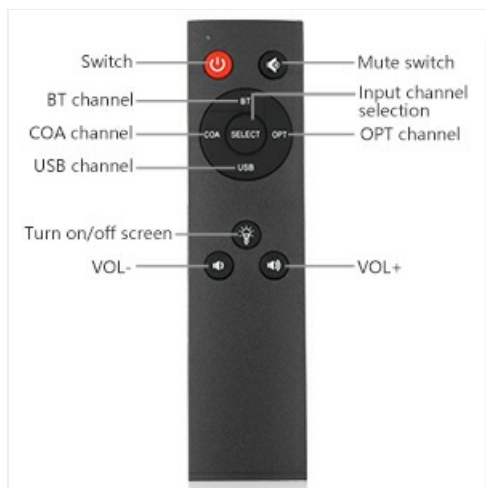
Image: Layout of the AIYIMA DAC A6 remote control, showing buttons for power, mute, input selection (BT, COA, OPT, USB), screen on/off, and volume up/down.
