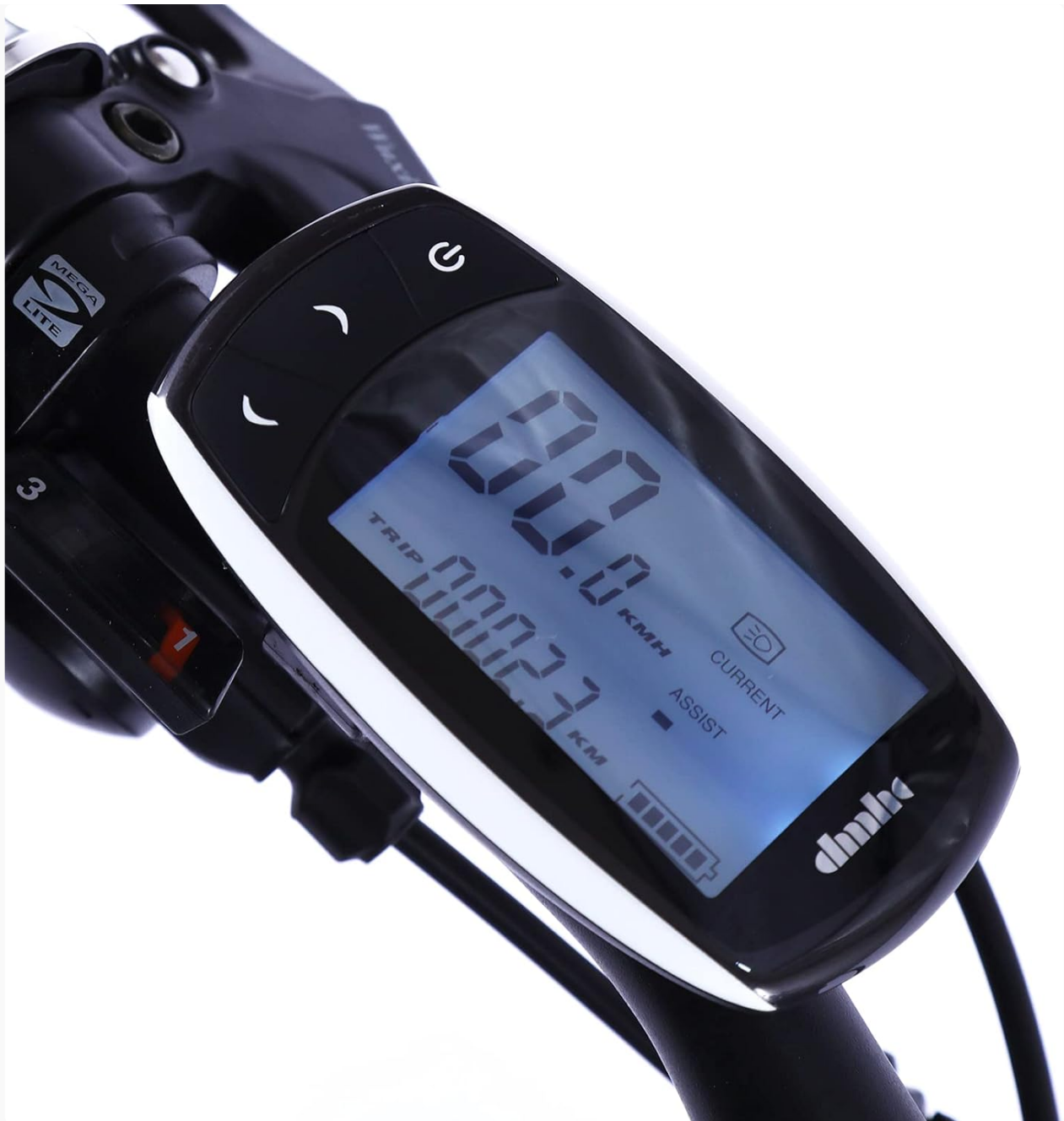
Figure 3.5: Close-up of the LCD display unit on the handlebars. The display shows current speed, trip distance, and battery charge level.
