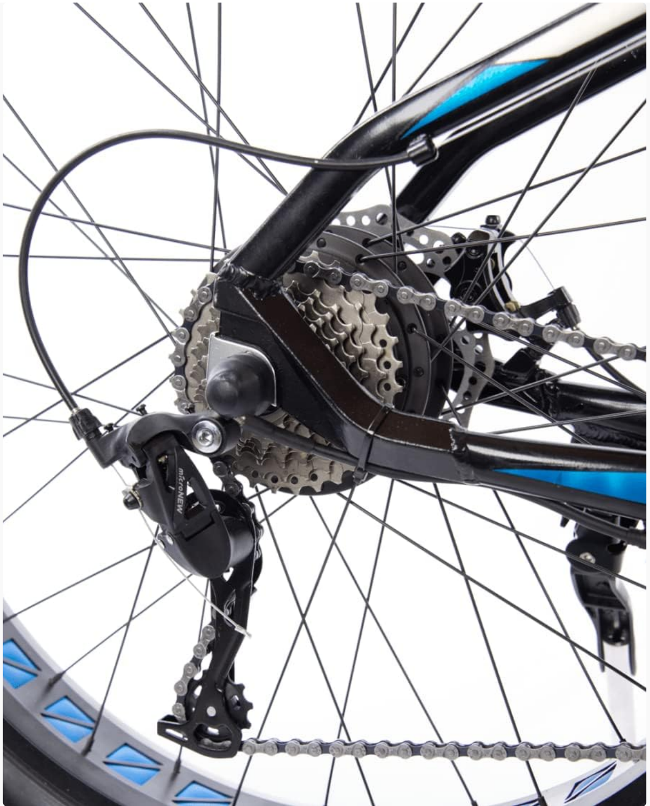
Figure 3.6: Close-up of the rear derailer and cassette. This image shows the multi-speed gearing system for varied terrain.
