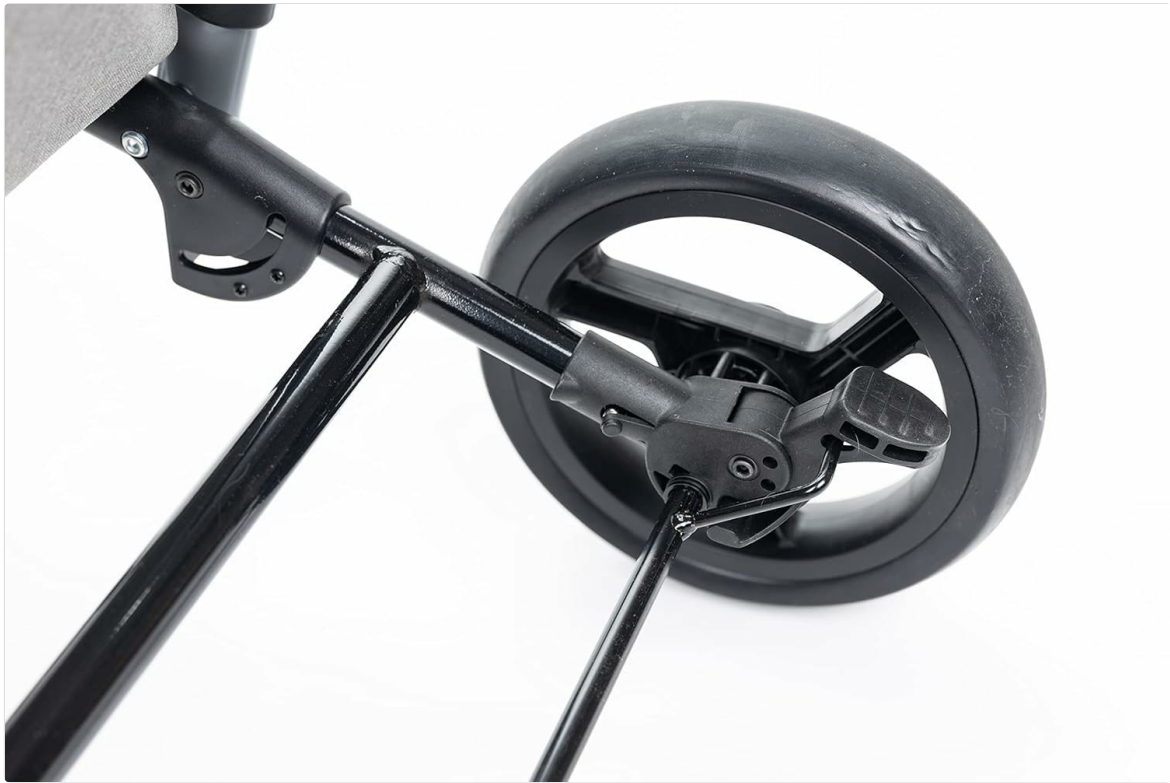
Image: Close-up of the rear wheel brake, showing the lever in the engaged position.
