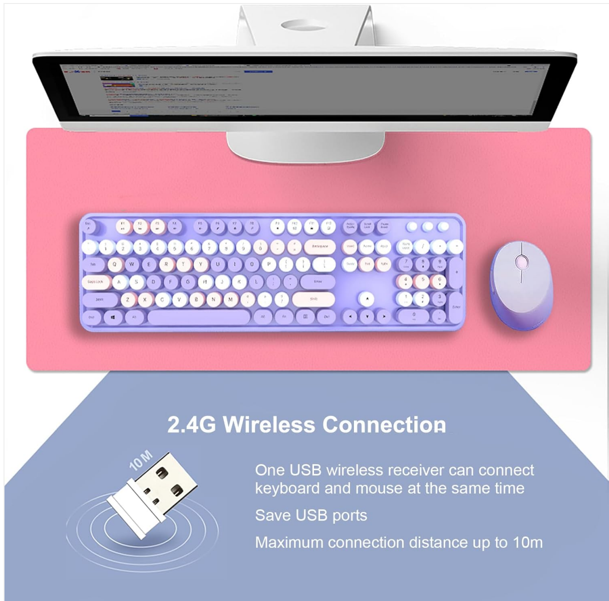
Image: A close-up of the USB receiver, illustrating its function for 2.4G wireless connection.
