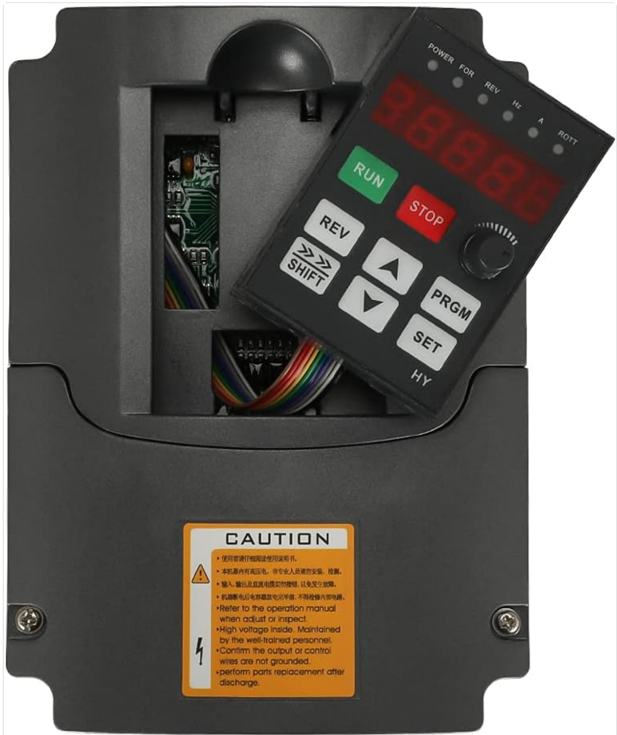
Figure 2: Front panel with display and control buttons, showing internal access.
