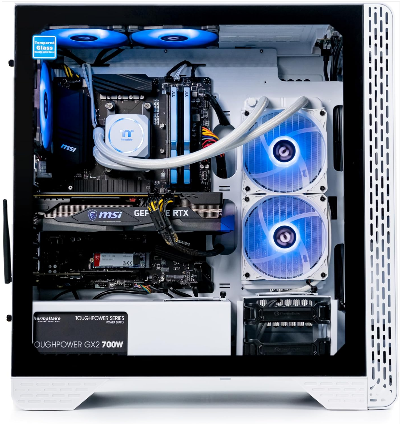
Image 1.2: Internal view of the Thermaltake Glacier 360 PC, showcasing the liquid cooling system, RAM, and graphics card.
