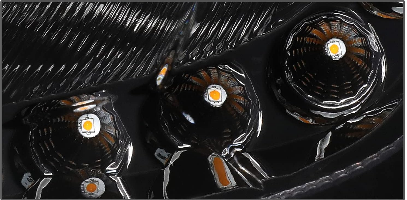
Image: Headlight demonstrating the sequential LED amber turn signal.
