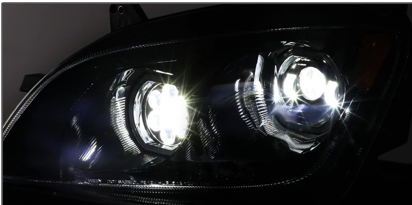
Image: Close-up of the full LED high beam and low beam in operation.
