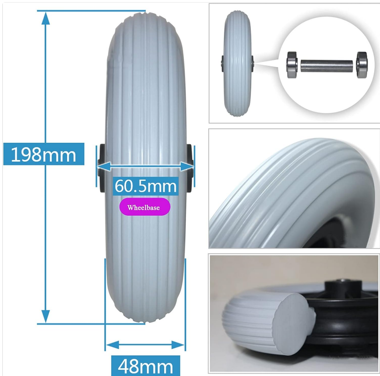
Figure 4: Dimensional diagram of the wheel, indicating a diameter of 198mm, a wheelbase of 60.5mm, and a width of 48mm.
