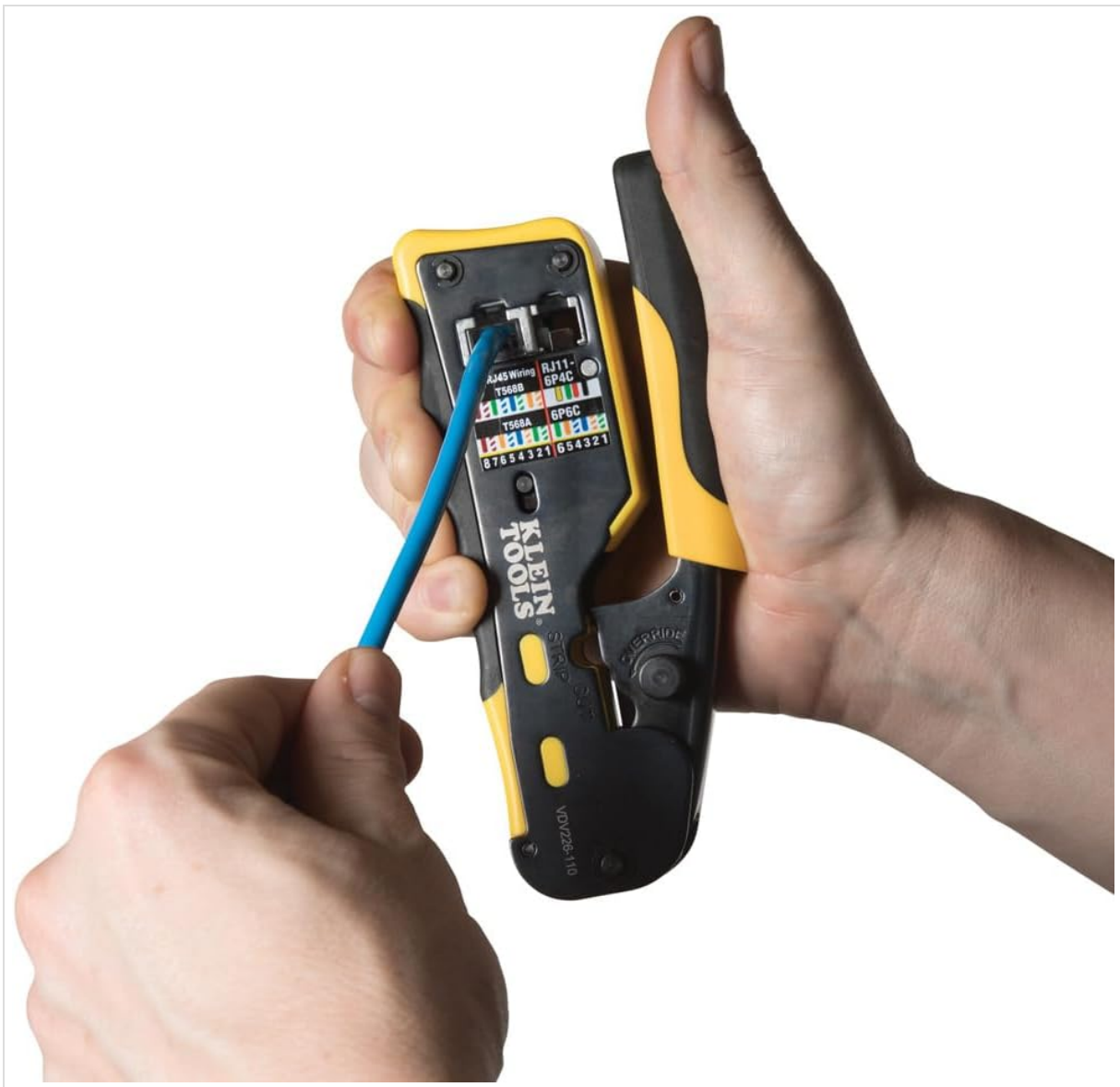
Image 4.2: A detailed view of the Klein Tools crimp tool's body, highlighting the integrated wiring diagrams for T568A and T568B standards, which guide the user in correct wire sequencing for RJ45 connectors.
