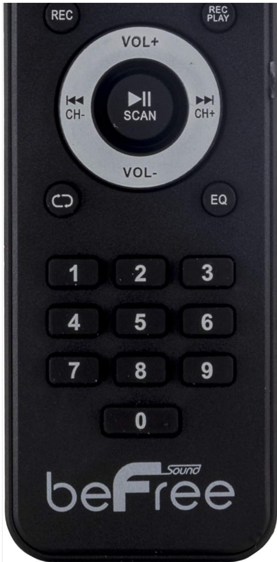
Figure 4.6: Remote Control. An image of the compact black remote control, featuring buttons for power, mute, mode selection, volume adjustment, track navigation, and equalizer settings.
