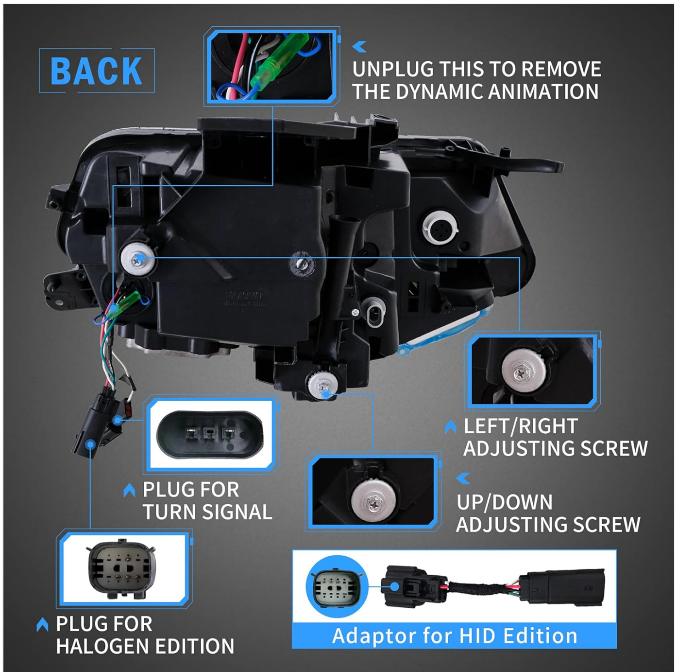
Figure 5.2: ACC plug connection for DRL function. Connect to the fuse box as shown for either HID or Halogen editions.
