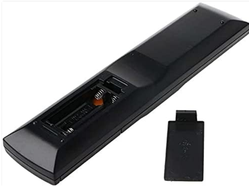
Figure 1: Back view of the remote control with the battery compartment open for battery installation.
