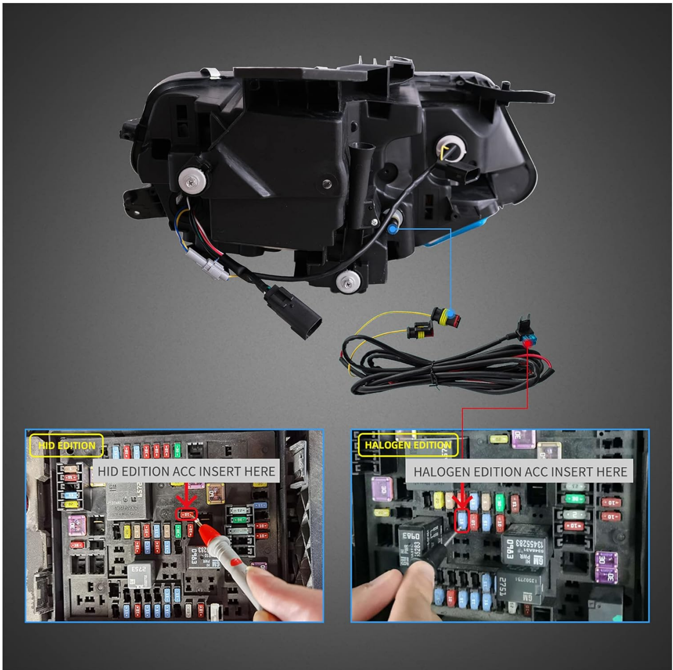
Image 4.2: Fuse box connection points for HID and Halogen editions.
