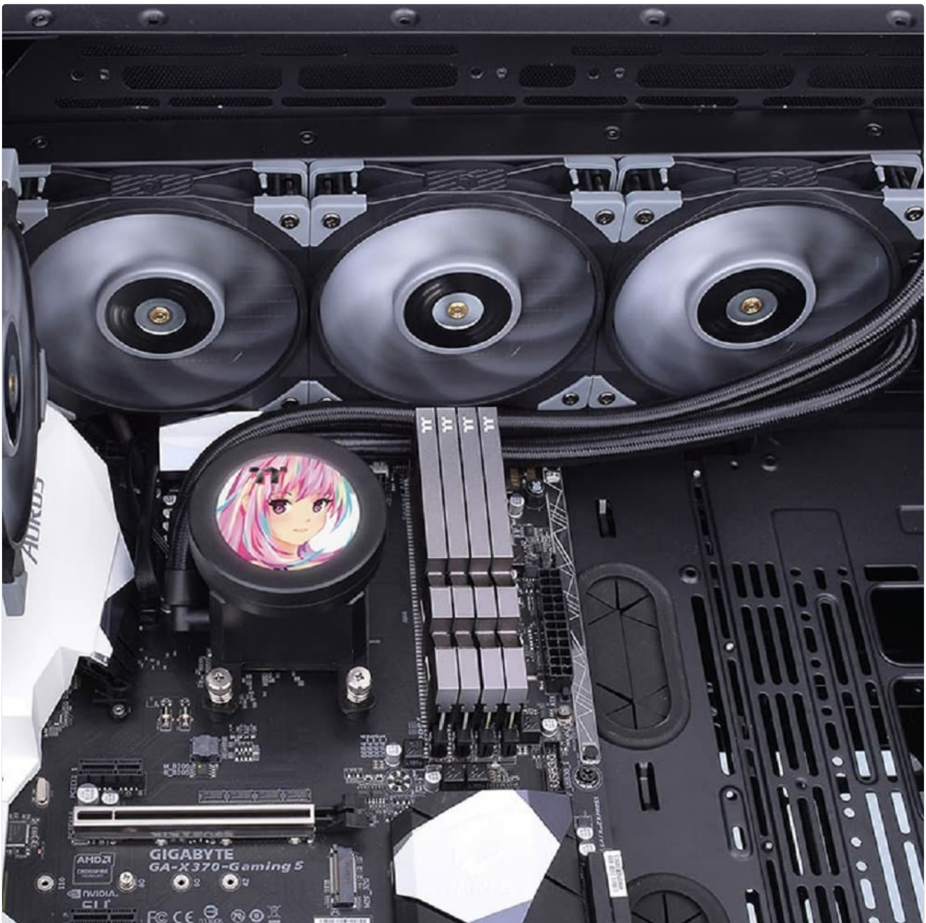
Image: The 2.1-inch LCD display on the water block, showing system information within a PC build.
