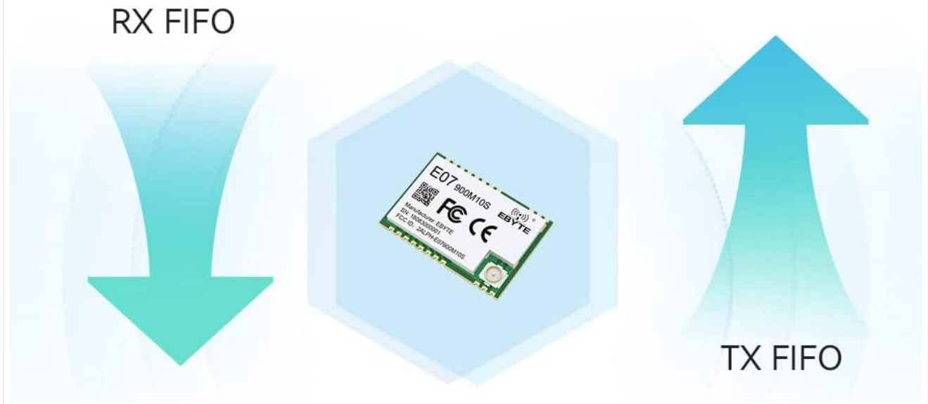
Figure 2.3: Illustration of the independent 64-byte Receive (RX) and Transmit (TX) FIFO buffers, which enhance data handling efficiency.
