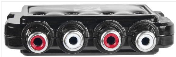
Figure 3: Side view of the NVX XMICROLOC4, clearly showing the four RCA output jacks. Two red jacks indicate right channels, and two white jacks indicate left channels for amplifier connection.
