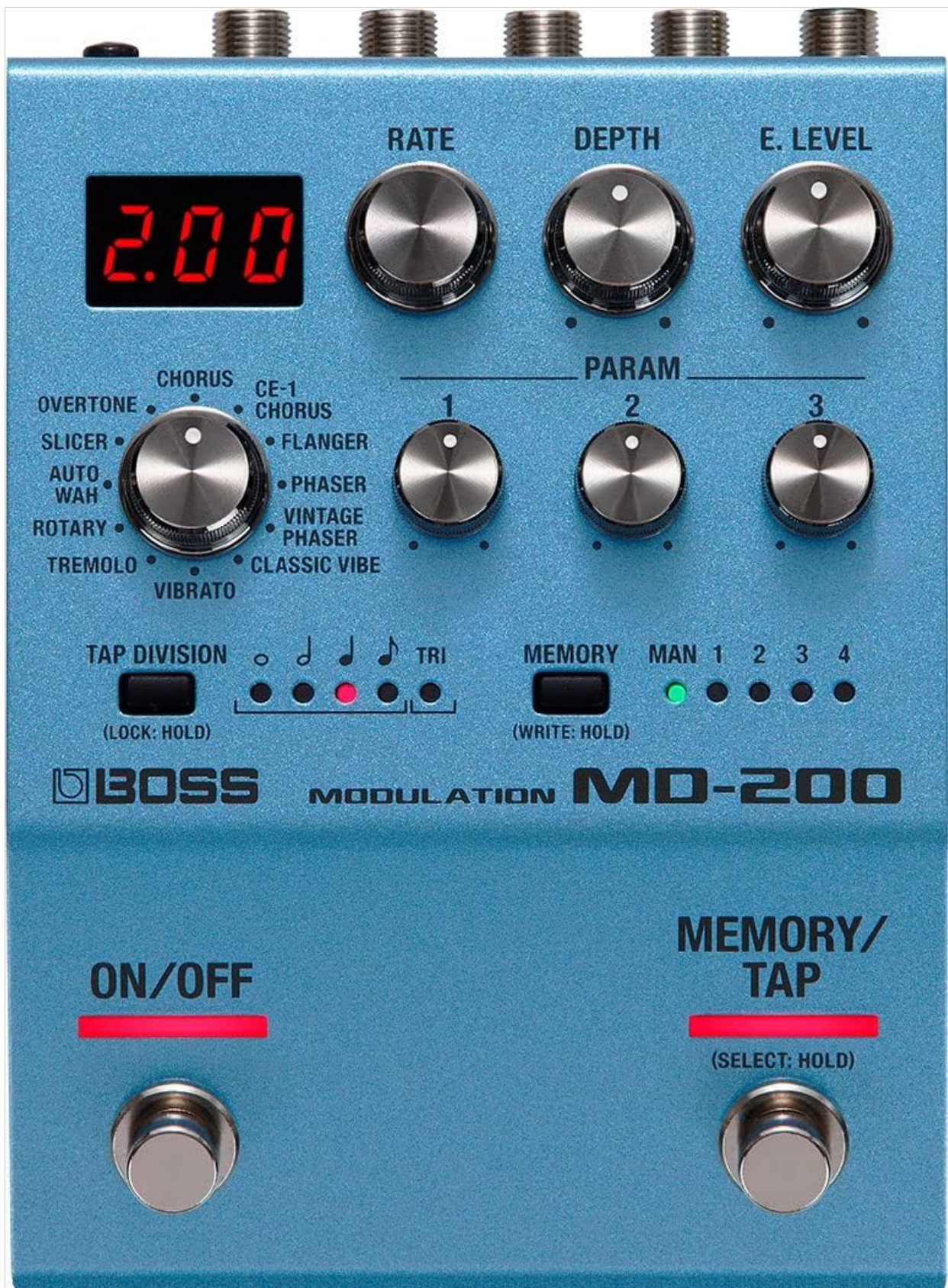
Figure 2: Front panel of the BOSS MD-200 Modulation Pedal, highlighting the display, control knobs, mode selector, and footswitches.
