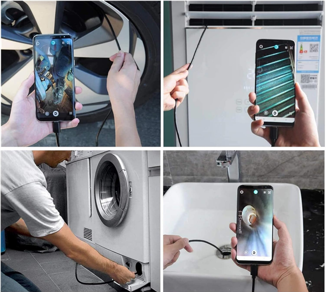
Image: Examples of the endoscope camera in use, showing inspections inside a car wheel well, an air conditioning unit, behind a washing machine, and down a sink drain, all viewed on a connected smartphone.
