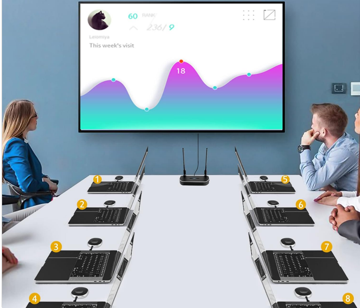
Image: A visual representation of the "Many-to-One Mode" where multiple transmitters can connect to a single receiver, allowing for easy switching between sources.
