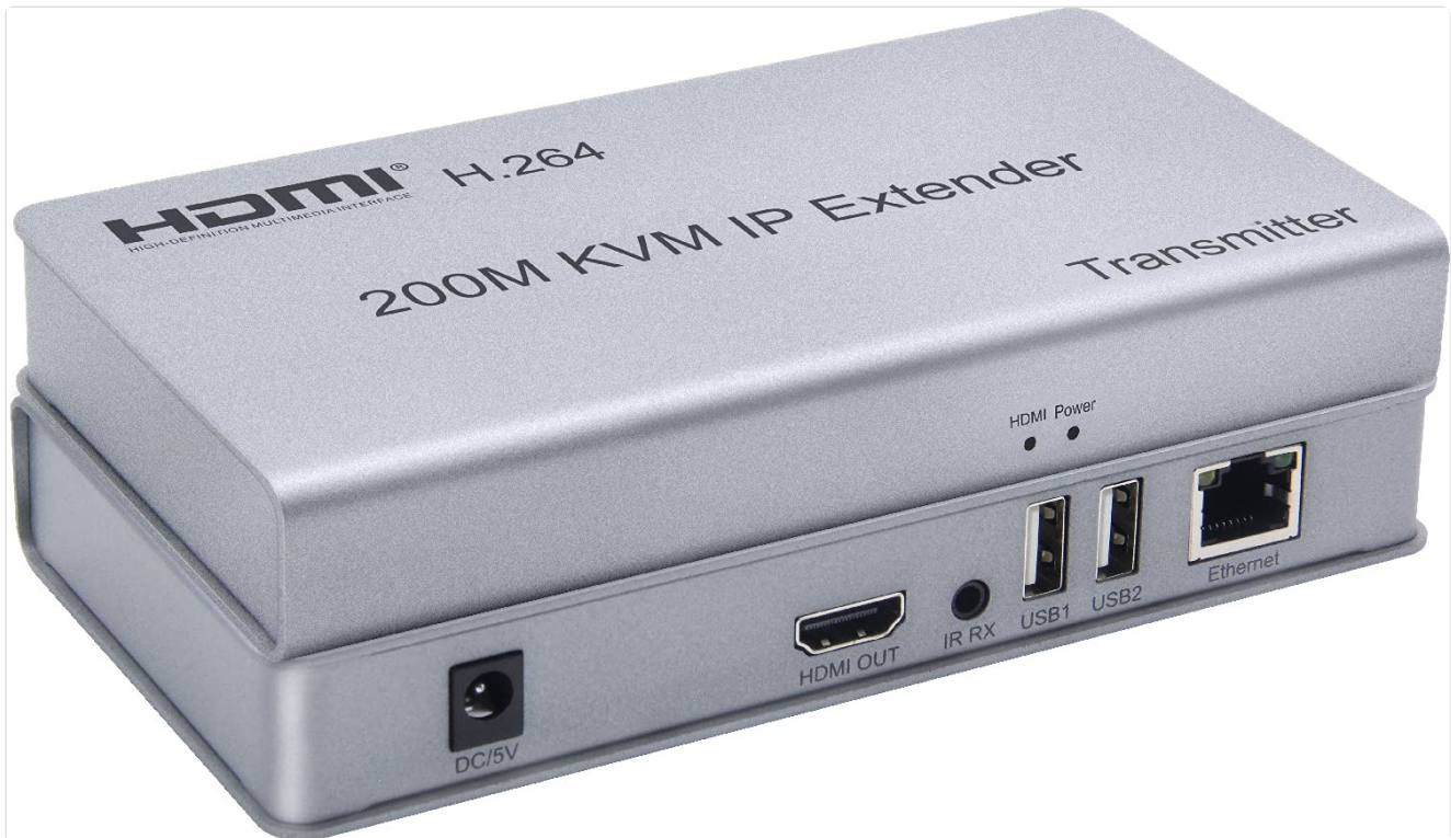
Figure 3.1: HDMI KVM IP Extender Transmitter (TX) Unit. This unit connects to the HDMI source and sends the signal over the network cable.
