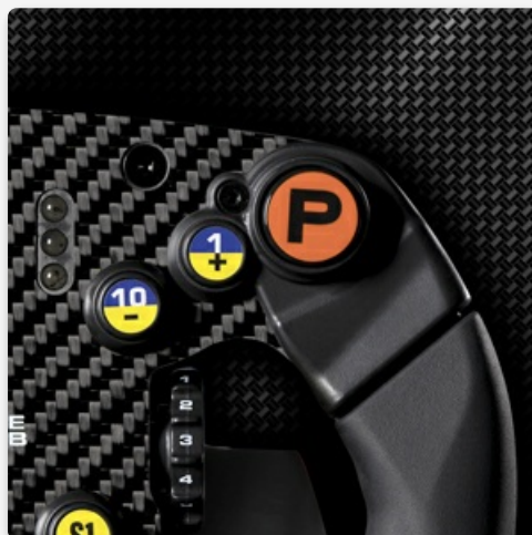
Image 5: The right side of the Ferrari SF1000 wheel, showing the 'P' (Pit Limiter) button and rotary encoders for incremental adjustments (+1, -10).
