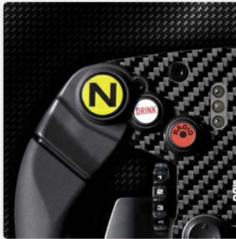
Image 4: The left side of the Ferrari SF1000 wheel, highlighting the 'N' (Neutral) button, 'DRINK' and 'RADIO' buttons, and a multi-position switch.
