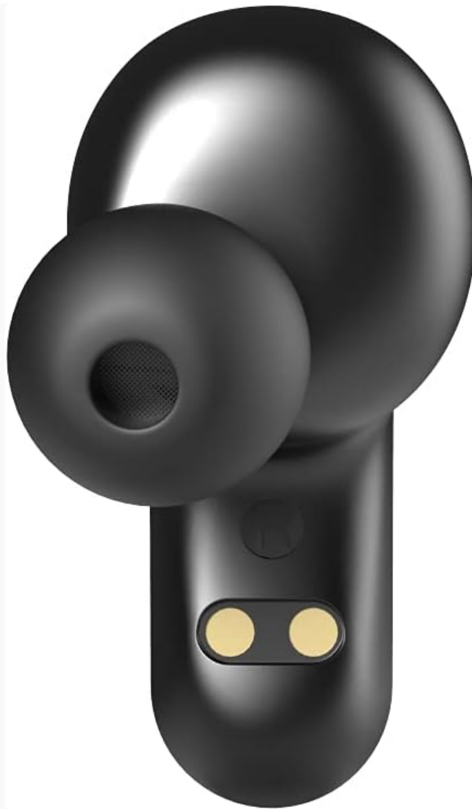
Image 5.1: A detailed view of the earbud's tip and charging contacts, showing areas that may require cleaning.
