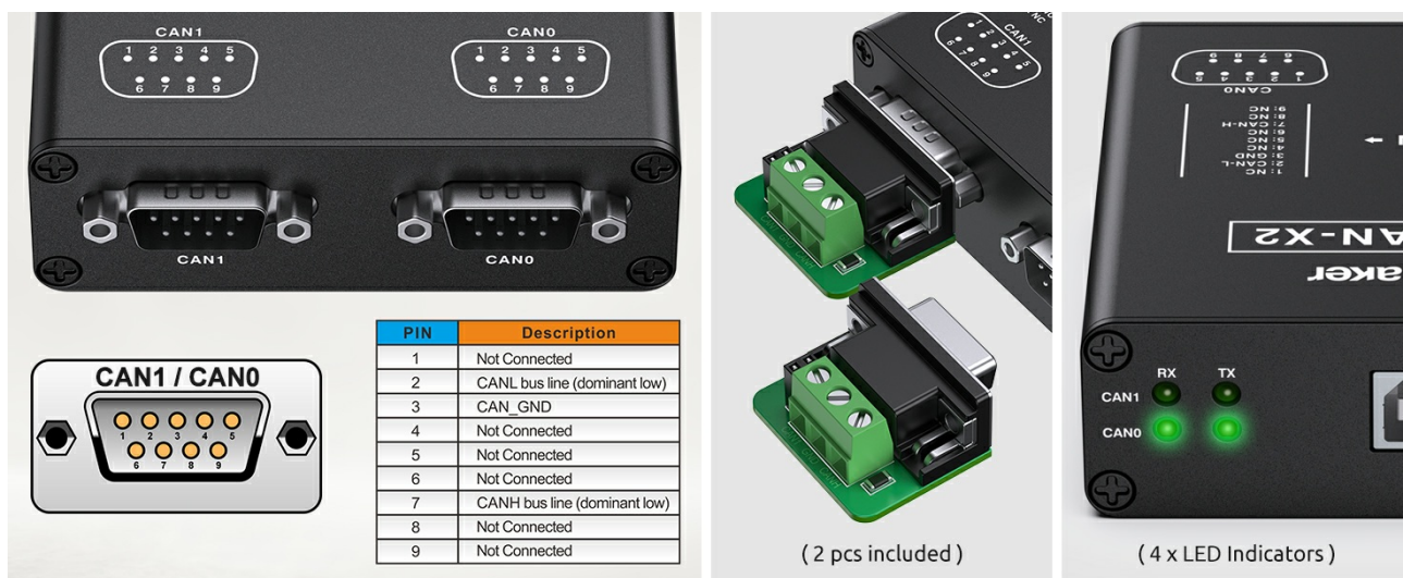
Figure 2.3: Detailed view of the USB2CAN-X2 showing the DB9 pinout for CAN1 and CAN0, along with the RX and TX LED indicators for each channel.
