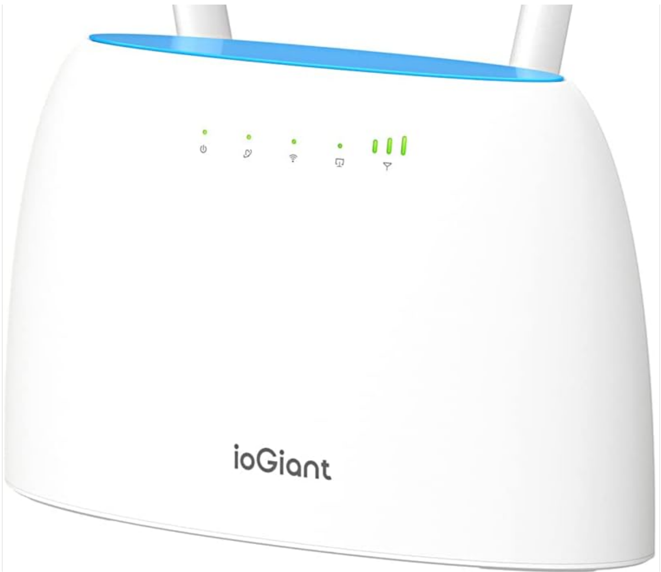
Figure 1: ioGiant AC1200 4G Router. This image shows the front of the router with its two external antennas and LED indicators.
