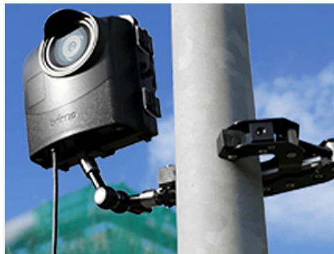
Image 3.3: Brinno camera in its waterproof housing securely mounted on a pole.
