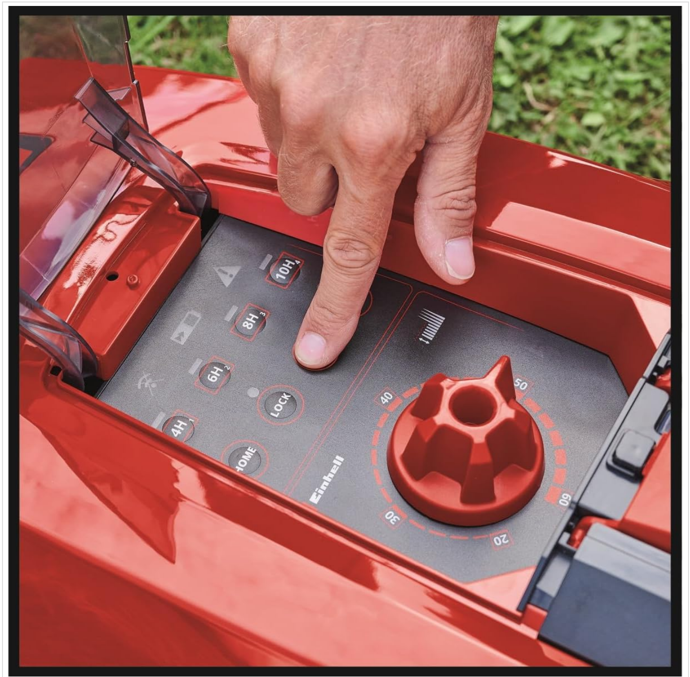
Figure 5: Close-up of the Einhell FREELEXO 350's control panel. This image shows the buttons for setting mowing times (e.g., 4H, 6H, 8H, 10H) and the central dial for cutting height adjustment.
