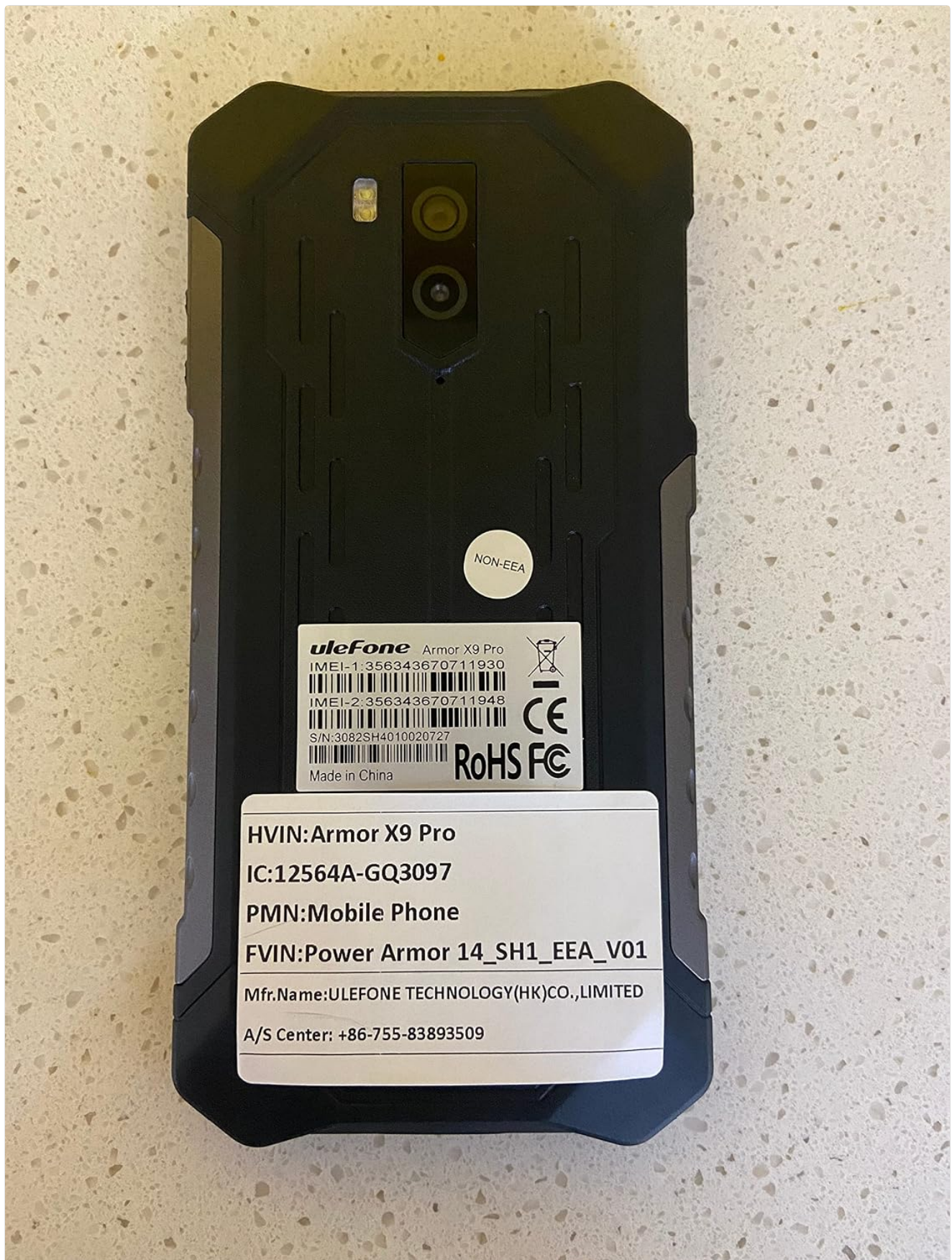
Figure 3.1: Rear view of the Ulefone Armor X9 Pro, highlighting the dual camera setup, LED flash, and regulatory information labels.
