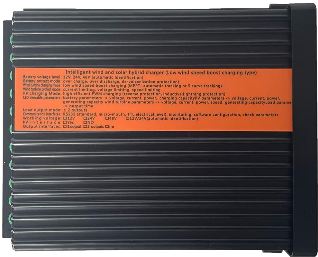
Figure 3.3: Top view of the controller, featuring a label with detailed specifications and operating modes.
