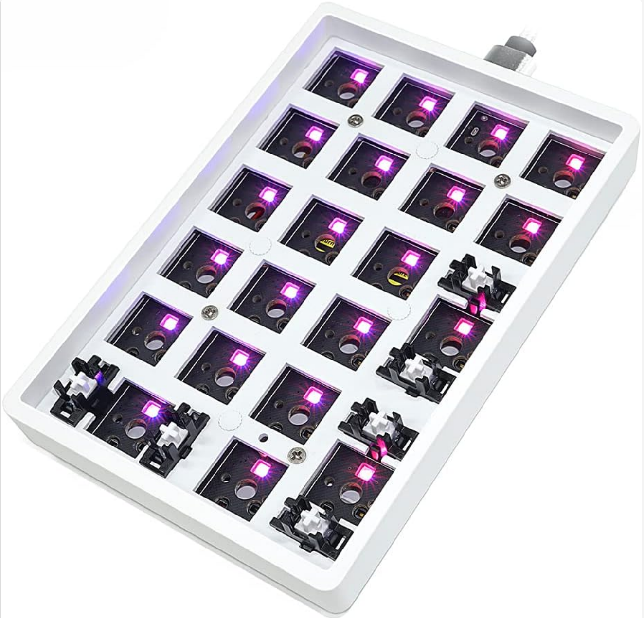
Image: The GK21S numpad kit showing the hot-swappable sockets ready for switch installation. The illuminated RGB LEDs indicate power is supplied to the PCB.
