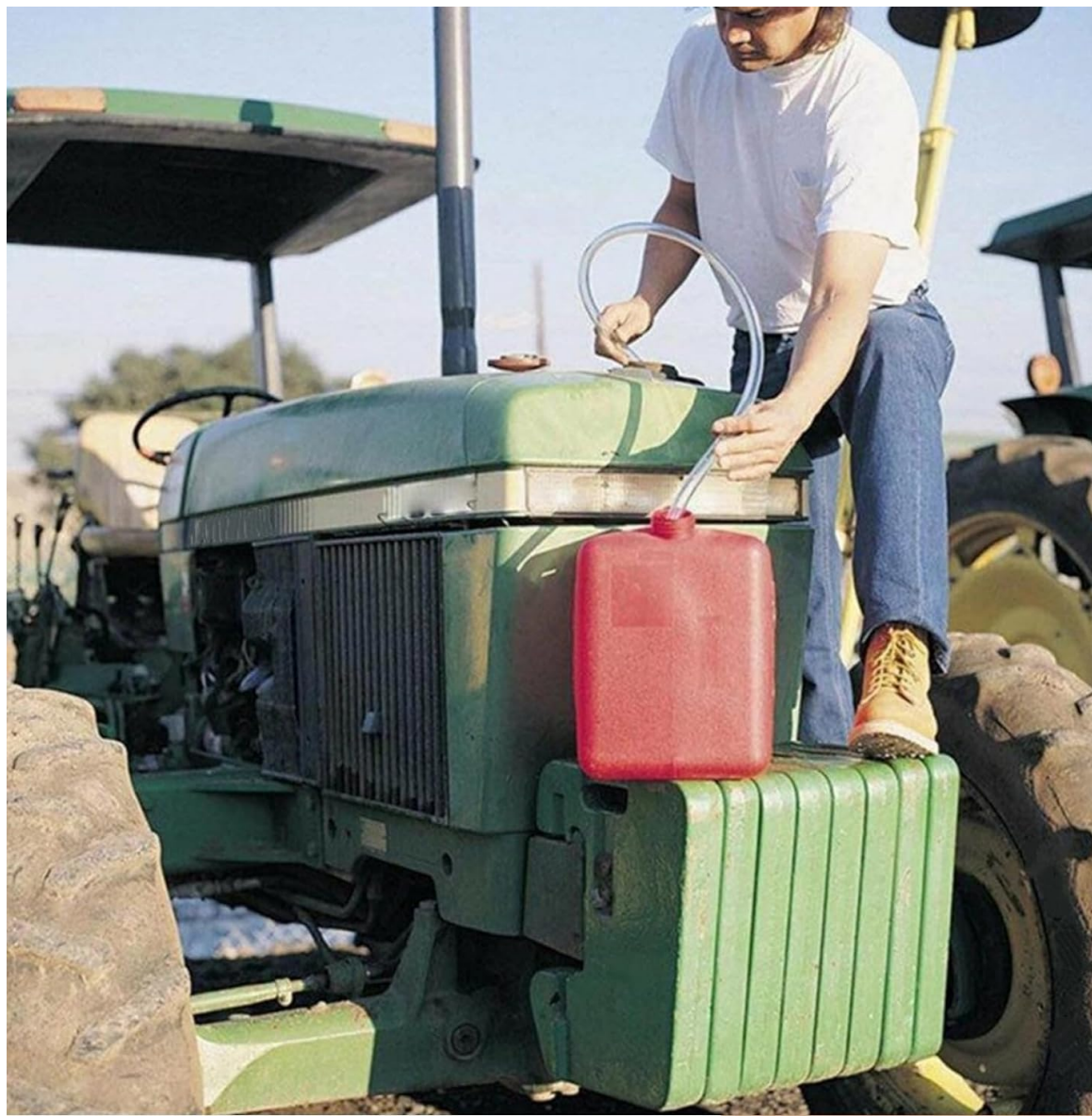
Image: A man using the siphon hose to transfer fuel from a tractor's tank into a red fuel can, illustrating a practical application.
